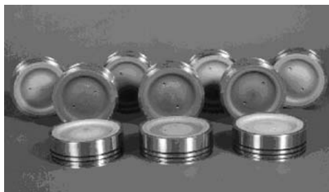
Fig. 5 As-sprayed HVOF coated steel pistons with various metallurgical protective coatings before use in diesel engines (left). Partially cleaned HVOF chromium-molybdenum-base coated steel piston after the use in a (stationary) ship diesel engine with increased fuel injection angle showing no wear, erosion, or corrosion damage or coating delamination (right)
